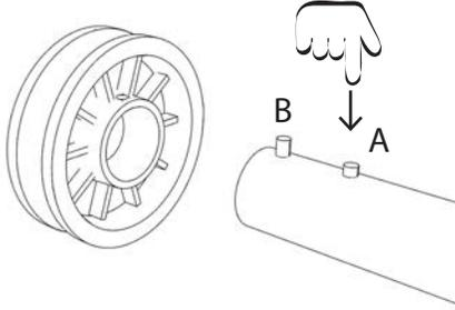
1.2. Line up pin (B) with hole in disc, insert rail into disc. Let pin (A) go.
