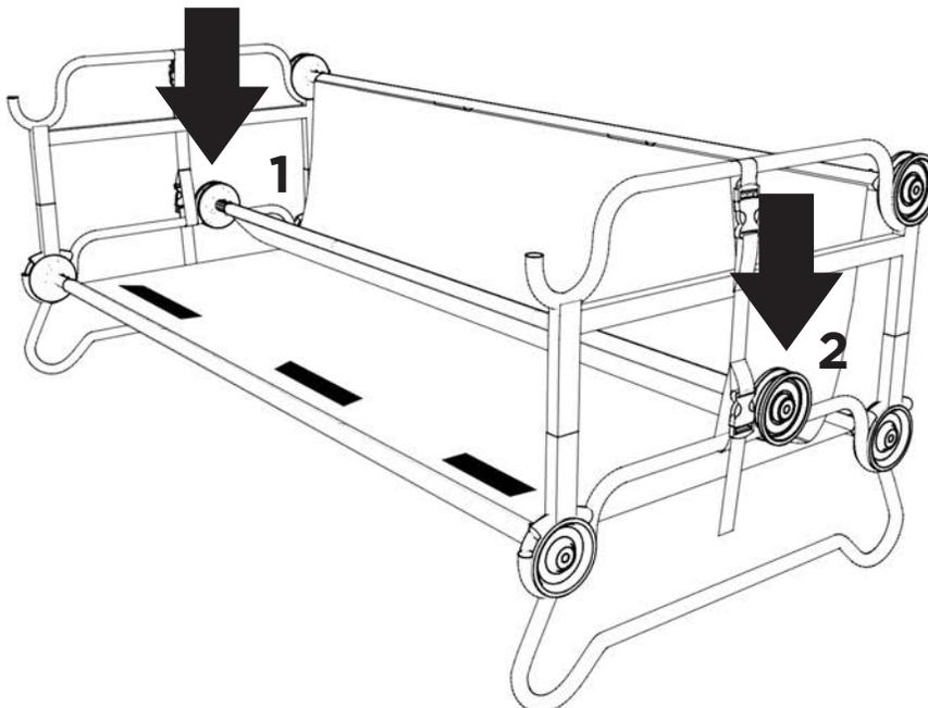
1.3 Let disc rest between bed end rail and stack adapter. The disc should not be able to roll forward.
